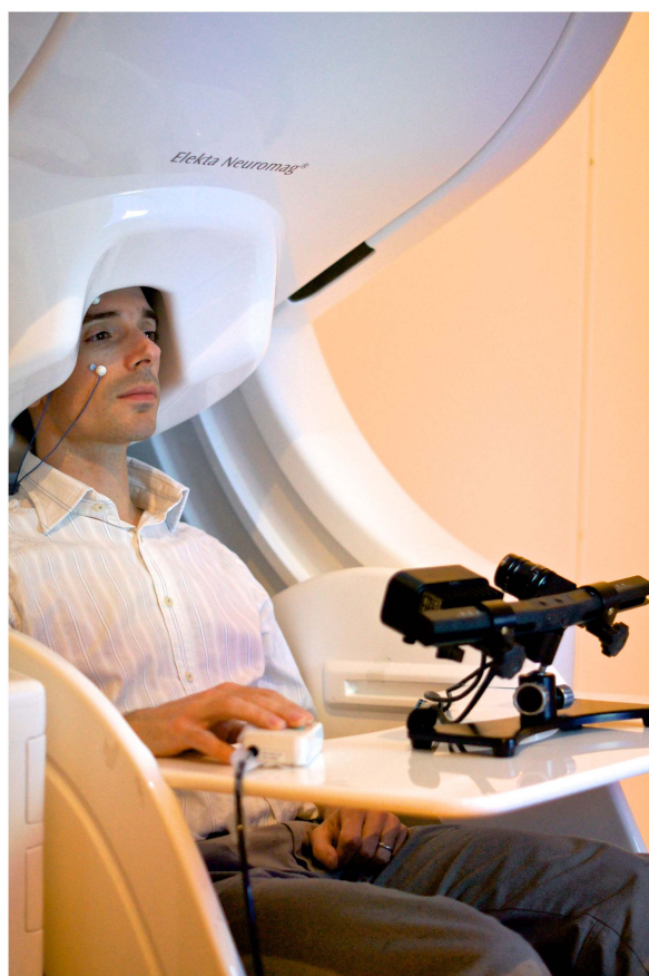
Figure 4 A MEG recording session at OHBA, eyetracker device shown in foreground.
