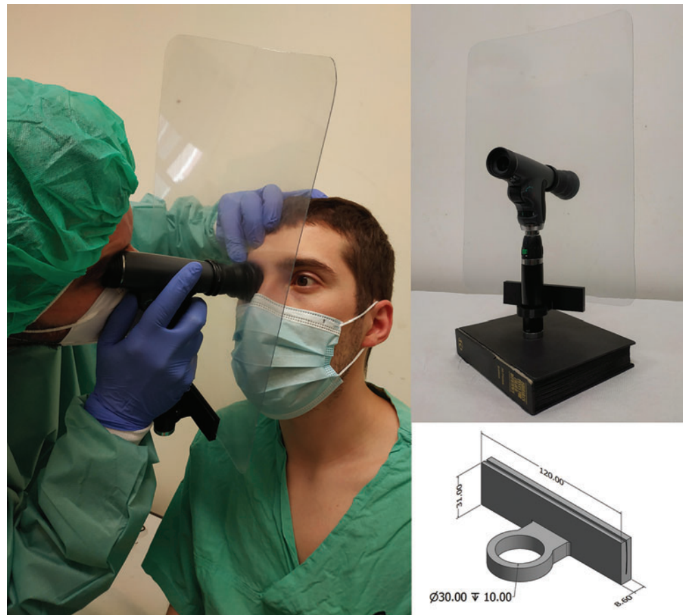
Figure 1 Ophthalmoscope protective shield. The protective shield (left and right upper segments) comprises three elements: (1) a plexiglass sheet (37×26 mm, 0.6 mm thickness) with a central hole (32 mm diameter), (2) two rubber rings (O-rings, 31 mm inner diameter) encircling the ophthalmoscope's head on each side of the sheet hole, (3) a three-dimensional printed polylactic acid component (right lower segment) docked around the power source/grip and attached to the lower border of the sheet to increase stability. The dimensions presented in computer-aided design model are in millimetres (right lower segment). We are currently making developments to the polylactic acid component to accommodate power handles of different sizes and simultaneous use of a charger.
