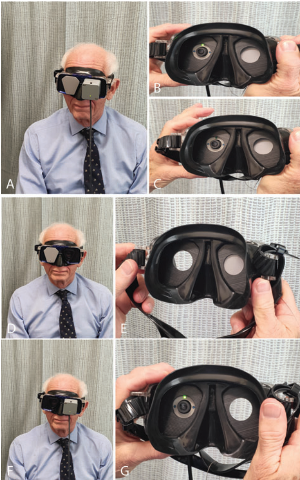
Figure 4 Infrared video nystagmus goggles. Camera with fixation LED occupies the left socket and cover occupies the right. (A) Examiner's view with fixation LED on. (B) Subject's view with fixation on. (C) Subject's view with fixation off—the subject would now be in total darkness. With camera out, cover in: (D) examiner's view; (E) subject's view; the subject can see the room. With camera in, fixation on, cover out: (F) examiner's view; (G) subject's view—the subject can also see the room.
