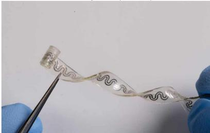
**Figure 1** Soft, bioresorbable coolers for reversible conduction block of peripheral nerves. Photograph: Northwestern University/PA.
