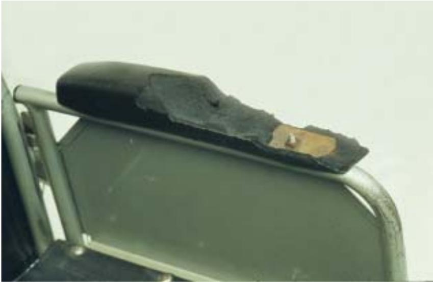
**Figure 8** Older wheelchair with eroded armrest and exposed bolt.
