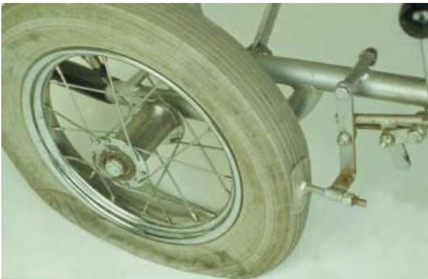
**Figure 4** Secondary brake failure – if the tyre is flat, the brake does not work.
