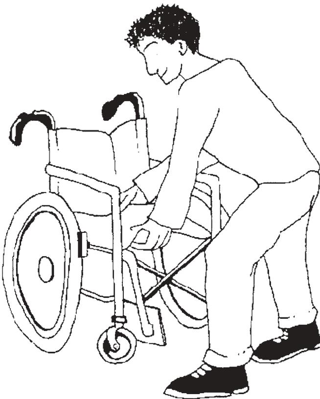
**Figure 9** How to fold a wheelchair. Lifting the centre of the canvas seat reduces the risk of finger trapping.
