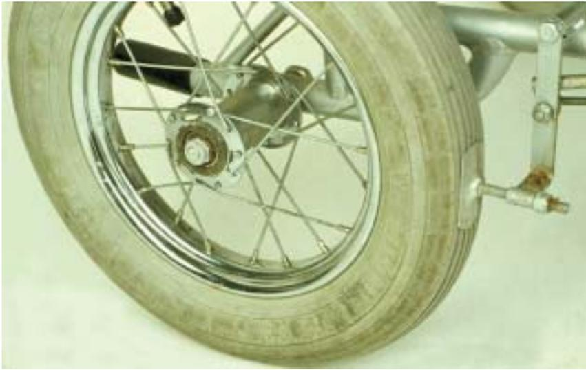
**Figure 3** The brake mechanism – a metal plate is applied to the tyre rim.
